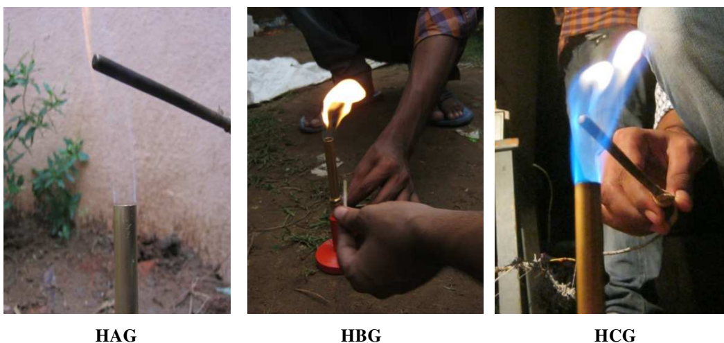
Figure 7: Photographic View of Flame Produced By Uncondensed Gas (HDPE)
